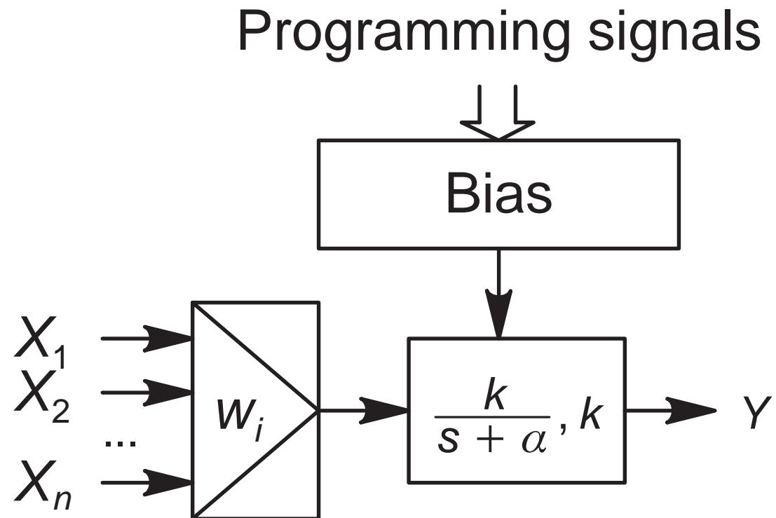
A straightforward implementation of the programmable integrator in OTA-C technique would lead to a switch in the signal path:
