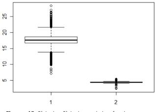
Figure 45 Side by Side box plots of axle space 1 (left) and 2(right)
