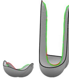
Fig. 5. Numerical predictions of critical wetting in corners with gaps using *Surface Evolver*: (left) slightly sub-critical, (right) super-critical.
