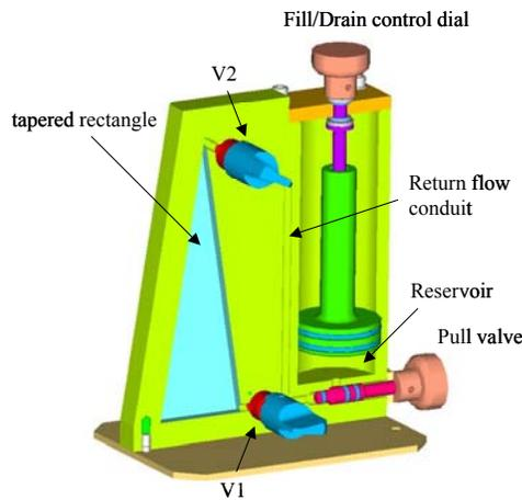
Fig. 1. ICF-2 tapered rectangular section.
