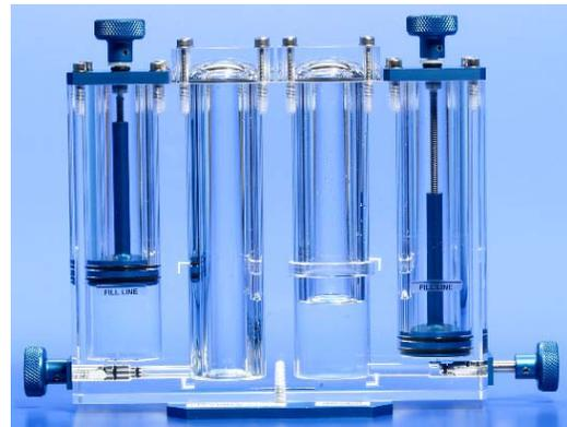
Fig. 7. Photograph of CL fluid-filled, prototype engineering unit. Left reservoir is filled, right test cell is filled.
