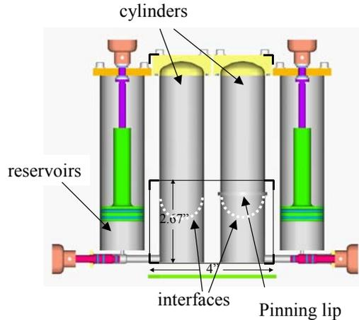
Fig. 6. Design for CL flight units with free and pinned contact lines. Dashed lines identify equilibrium menisci shapes in microgravity environment. The primary camera FOV is identified by the 4" by 2.67" window.
