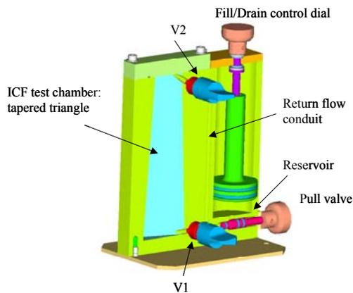
Fig. 1. ICF-1 tapered isosceles triangle section.
