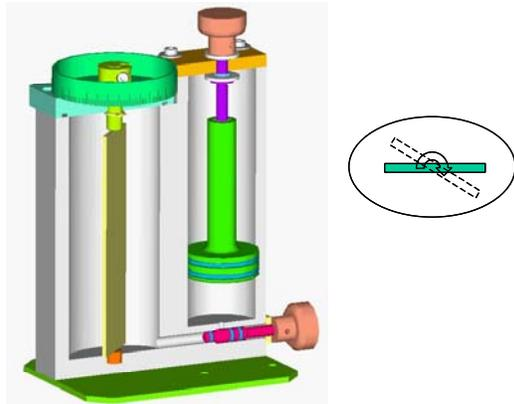
Fig. 4. VG flight unit with elliptical section and rotatable vane shown at right.
