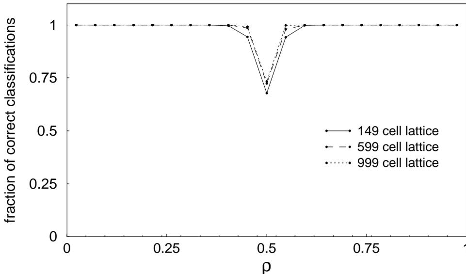
Figure 3: Experimental performance of the GKL rule as a function of  $\rho(0)$  for the  $\rho_c = 1/2$  task. Performance plots are given for three lattice sizes:  $N = 149$  (the size of the lattice used in the GA runs), 599, and 999.
