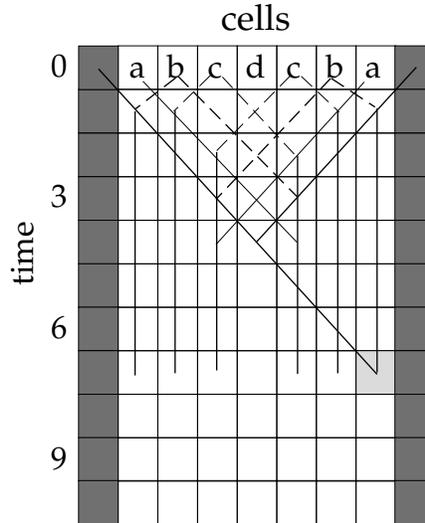
Figure 10: Schematic illustration of Smith’s  $r = 1$  bounded CA that recognizes the context-free language  $L_1$  (consisting of palindromes) in real time. The lightly shaded rightmost cell at  $t = 7$  indicates acceptance of the input.
