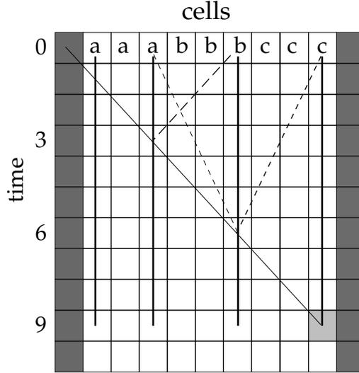
Figure 11: Schematic illustration of Smith’s bounded CA that recognizes the context-sensitive language  $L_2 = \{a^m b^m c^m \mid m \geq 1\}$  in real time. The lightly shaded rightmost cell at  $t = 9$  indicates acceptance of the input.
