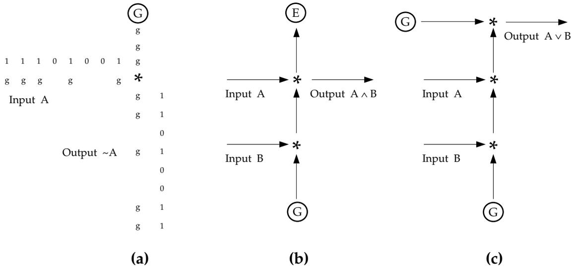
Figure 7: NOT (a), AND (b), and OR (c) gates built out of gliders (labeled  $g$ ), glider guns (labeled  $G$ ), and “eaters” (labeled  $E$ ) in Life. The symbol  $*$  indicates a glider collision. (Adapted from Berlekamp, Conway, and Guy, 1982.)
