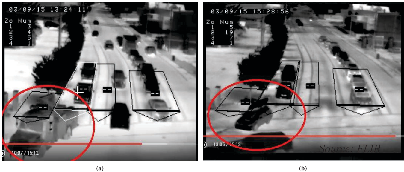
FIGURE 4 FLIR sources of false positives in right-turn lane: (a) trucks with protruding equipment and (b) cars with roof attachments.
