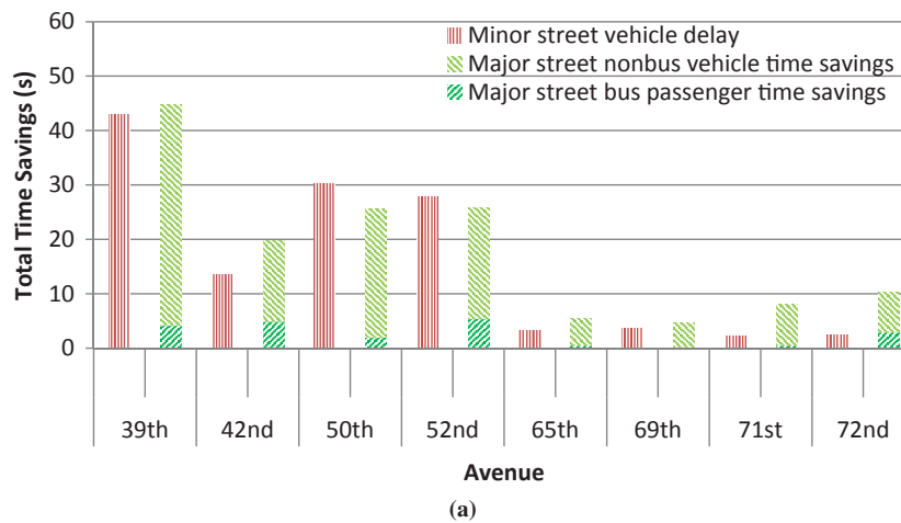
FIGURE 10 Total passenger time savings and vehicle delays per second of TSP phase: (a) GE.
