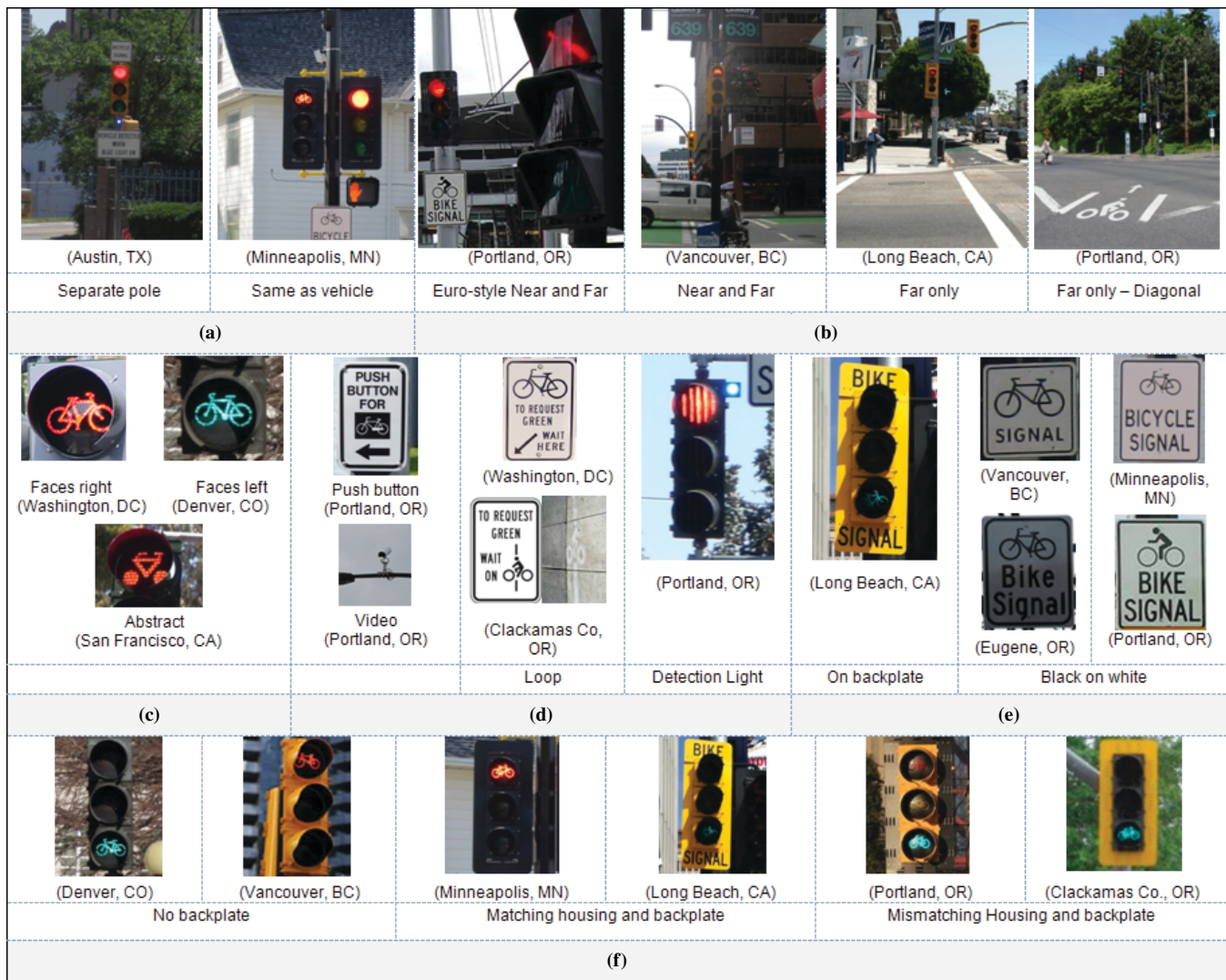
FIGURE 3 Various elements of bicycle-specific traffic signals: (a) mounting, (b) placement, (c) insignia, (d) detection, (e) signage, and (f) backplate and housing.
