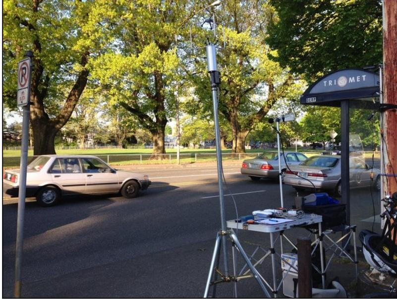
**Figure 5. Portable roadside air quality monitoring setup**
