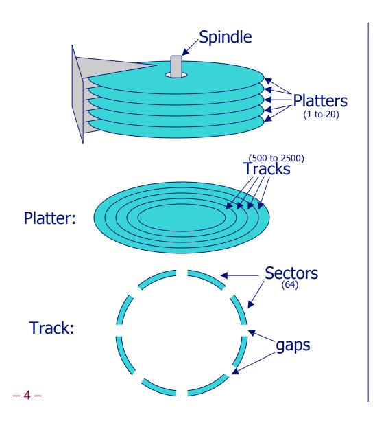
We shall stack 1 to 20 metal discs, each side covered with magnetic recording material, and bind them by a central spindle.
