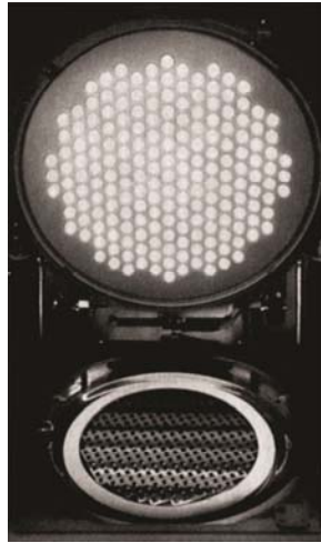
Figure 6.16 The Applied Materials Centura RTP Honeycomb source in the lifted position. The wafer is in the lower part of the photograph ( courtesy Applied Materials ).
