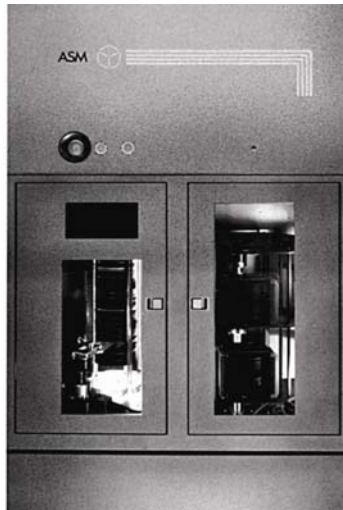
Figure 4.26 Vertical oxidation system showing carousel, robot arm, and wafers about to be raised into the furnace (photo courtesy of ASM International).
