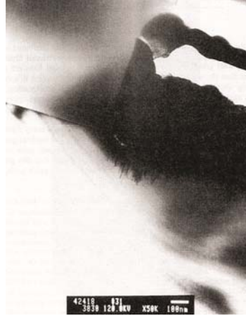
Figure 13.25 Damage to the substrate produced by selective tungsten.
