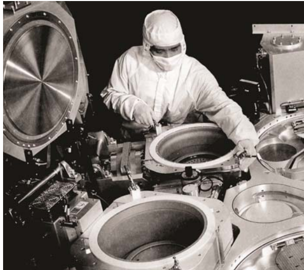
Figure 12.25 The Endura system by Applied Materials uses a number of PVD or CVD chambers fed by a central robot. For conventional and IMP (ionized metal plasma) sputtering, targets are hinged to open upward. Two open chambers are shown, along with the load lock (from Applied Materials).
