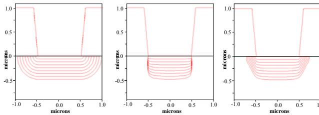
a). all chemical etching (ion flux=0); b). all physical or ionic etching (chem flux=0); c). half chemical, half physical.
