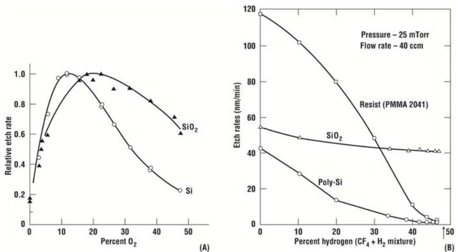
**Figure 11.12** Etch rate of Si and SiO<sub>2</sub> in (A) CF<sub>4</sub>/O<sub>2</sub> plasma (after Mogab et al. [59], reprinted by permission, AIP), and (B) CF<sub>4</sub>/H<sub>2</sub> plasma (after Ephrath and Petrillo [100], reprinted by permission of the publisher, The Electrochemical Society Inc.)
