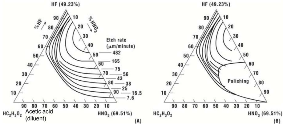
**Figure 11.4** The etch rate of silicon in HF and HNO<sub>3</sub> (after Schwarz and Robbins, reprinted by permission of the publisher, The Electrochemical Society Inc.).
