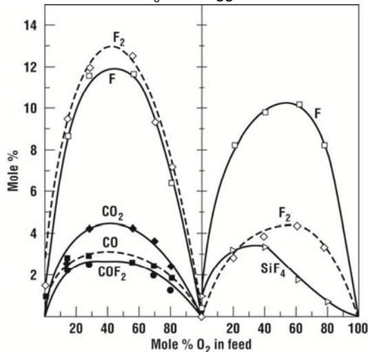
**Figure 11.10** Species concentration in a CF<sub>4</sub> plasma as a function of the amount of oxygen in the feed gas (after Smolinsky and Flamm, reprinted by permission, AIP).
