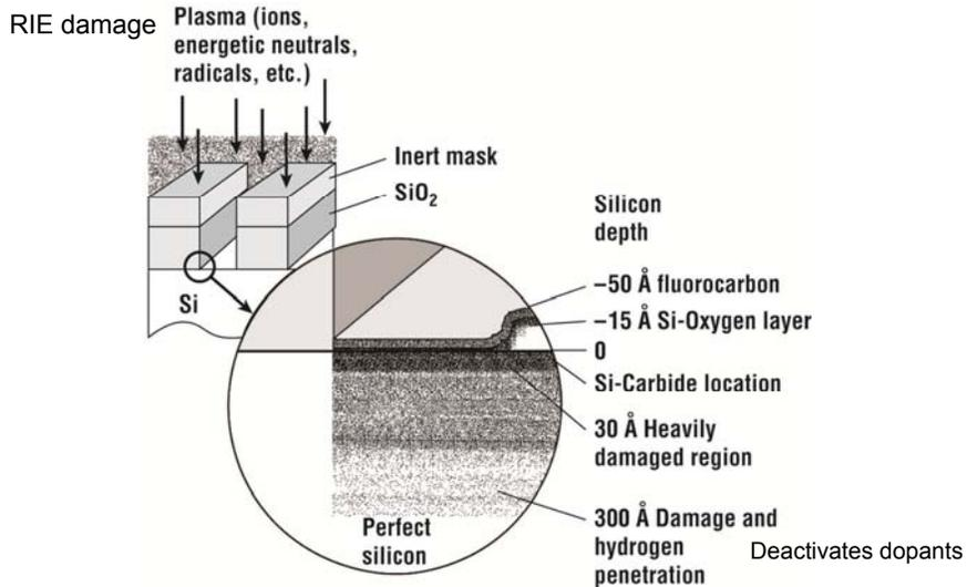
**Figure 11.21** A cross section schematic of the results of a typical etch of  $\text{SiO}_2$  down to Si using  $\text{CF}_4/\text{H}_2$  (after Oehrlein, Rembetski, and Payne, reprinted by permission, AIP).
