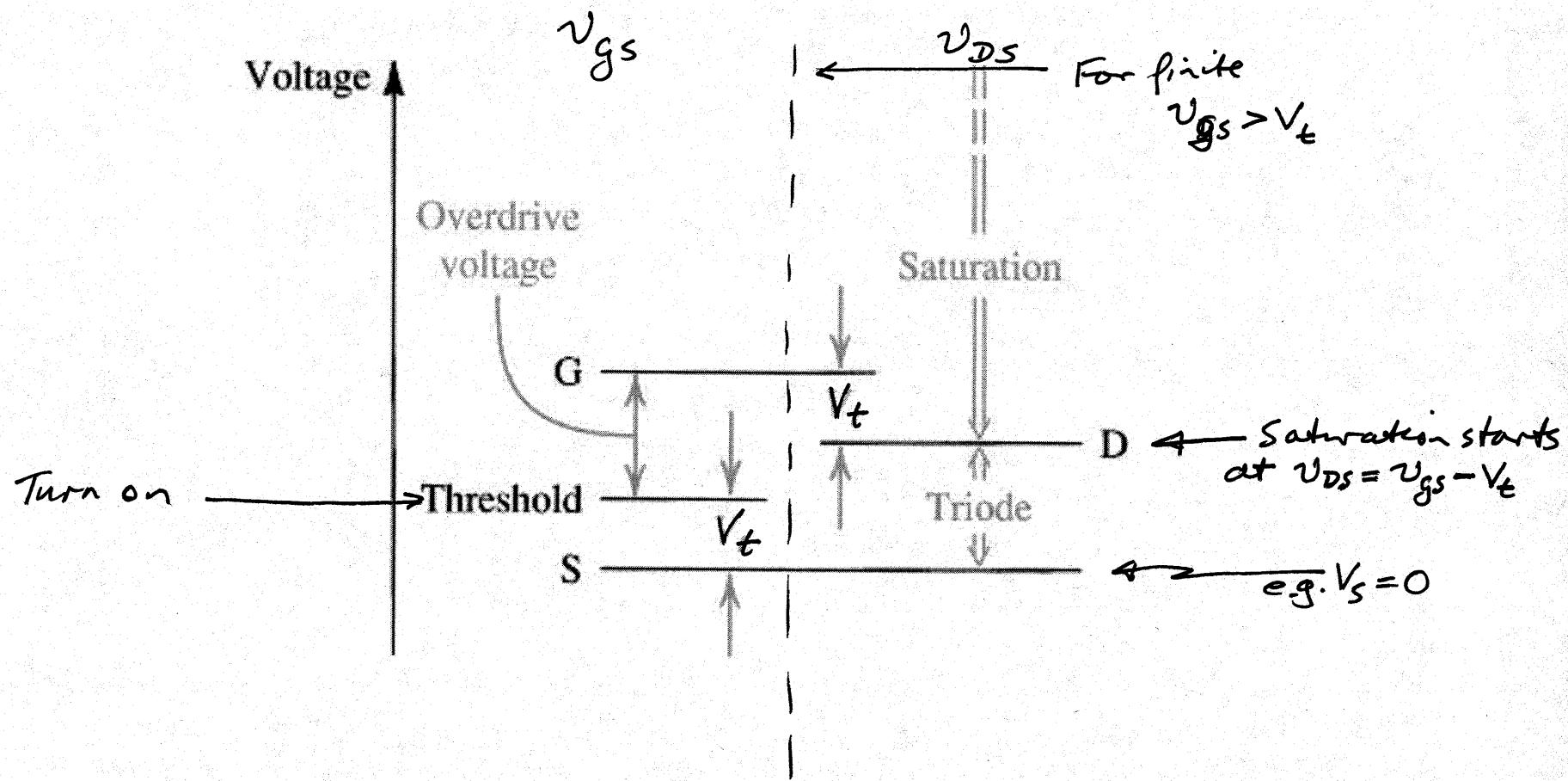
**Figure 4.14** The relative levels of the terminal voltages of the enhancement NMOS transistor for operation in the triode region and in the saturation region.
