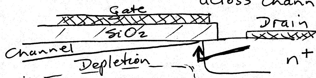
Figure 4.7 Increasing  $v_{DS}$  causes the channel to acquire a tapered shape. Eventually, as  $v_{DS}$  reaches  $v_{GS} - V_t$  the channel is pinched off at the drain end. Increasing  $v_{DS}$  above  $v_{GS} - V_t$  has little effect (theoretically, no effect) on the channel's shape.
