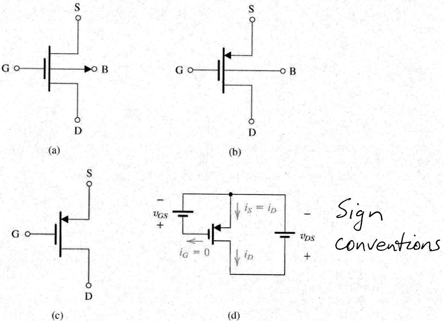
**Figure 4.18** (a) Circuit symbol for the *p*-channel enhancement-type MOSFET. (b) Modified symbol with an arrowhead on the source lead. (c) Simplified circuit symbol for the case where the source is connected to the body. (d) The MOSFET with voltages applied and the directions of current flow indicated. Note that  $v_{GS}$  and  $v_{DS}$  are negative and  $i_D$  flows out of the drain terminal.
