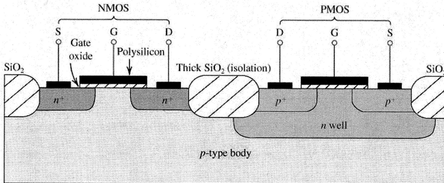
**Figure 4.9** Cross-section of a CMOS integrated circuit. Note that the PMOS transistor is formed in a separate  $n$ -type region, known as an  $n$  well. Another arrangement is also possible in which an  $n$ -type body is used and the  $n$  device is formed in a  $p$  well. Not shown are the connections made to the  $p$ -type body and to the  $n$  well; the latter functions as the body terminal for the  $p$ -channel device.
