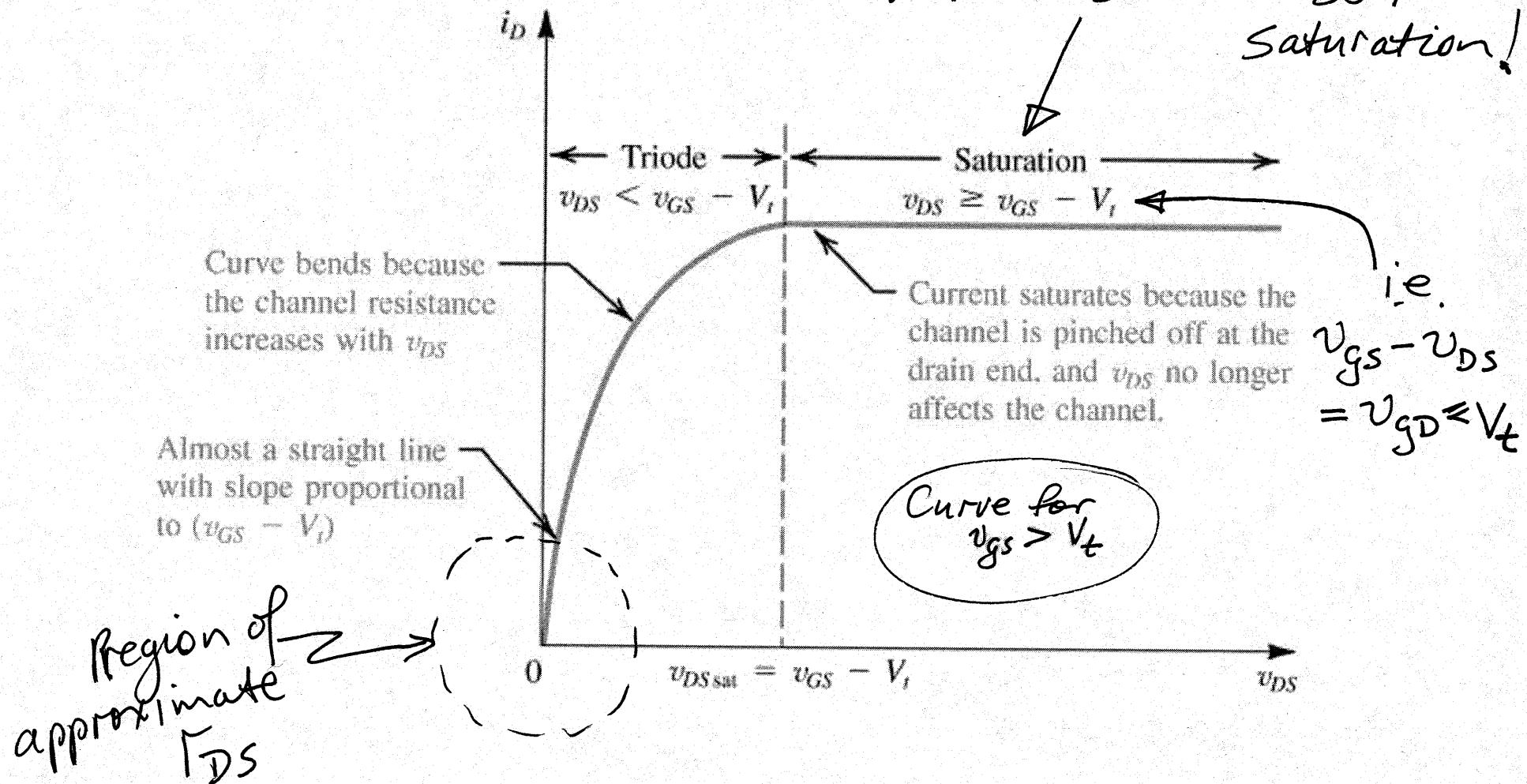
**Figure 4.6** The drain current  $i_D$  versus the drain-to-source voltage  $v_{DS}$  for an enhancement-type NMOS transistor operated with  $v_{GS} > V_t$
