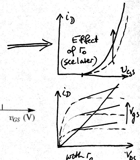
Figure 4.12 The  $i_D-v_{GS}$  characteristic for an enhancement-type NMOS transistor in saturation ( $V_t = 1$  V,  $k_n' W/L = 1.0$  mA/V<sup>2</sup>).
