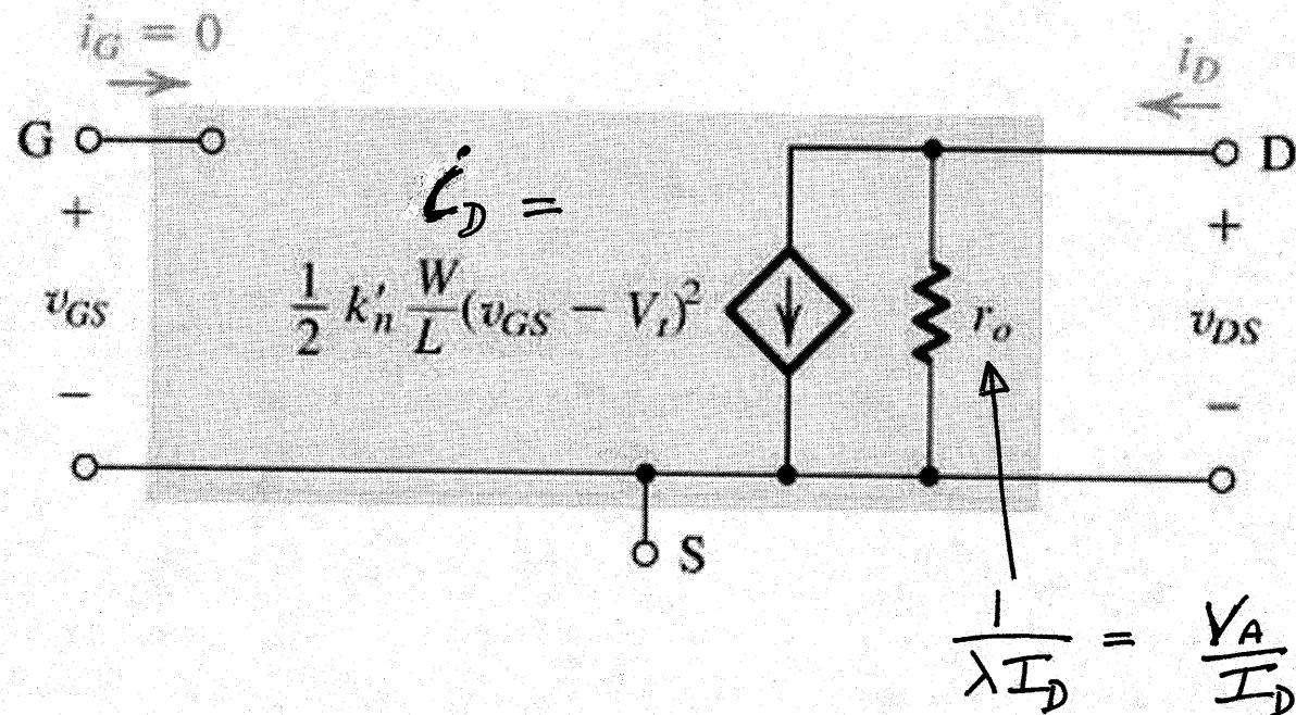
**Figure 4.17** Large-signal equivalent circuit model of the  $n$ -channel MOSFET in saturation, incorporating the output resistance  $r_o$ . The output resistance models the linear dependence of  $i_D$  on  $v_{DS}$  and is given by Eq. (4.22).
