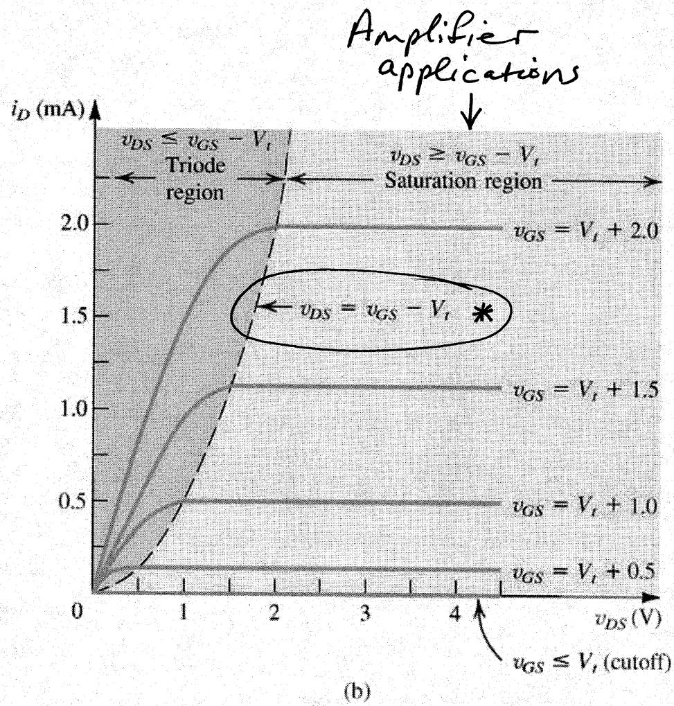
Figure 4.11 (a) An *n*-channel enhancement-type MOSFET with  $v_{GS}$  and  $v_{DS}$  applied and with the normal directions of current flow indicated. (b) The  $i_D$ - $v_{DS}$  characteristics for a device with  $k'_n(W/L) = 1.0 \text{ mA/V}^2$ .
