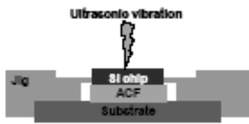
Figure 3. A schematic diagram of the flip chip assembly structure using a jig for TS bonding.
