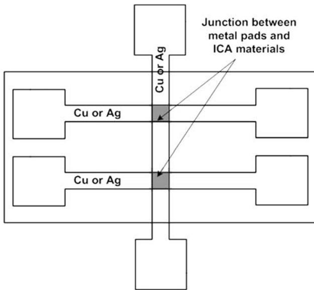
Fig 2 Schematic of a junction resistance test device
