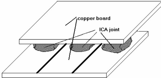
Figure 1 – Schematic Configuration A
