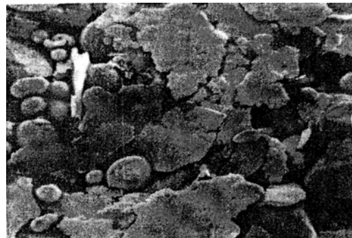
Figure 1 ICA bi-modal filler distribution (Ag flakes & powder), with surface layering evident.
