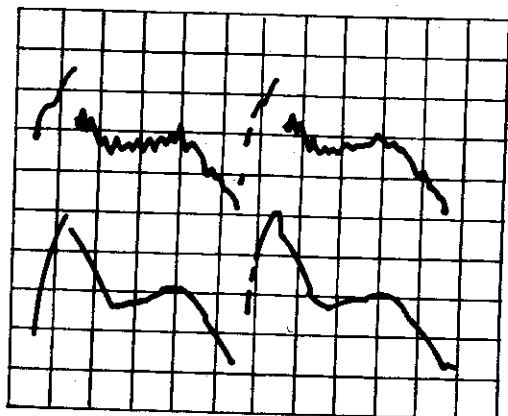
Figure 10. PLL #1 output v_{01} (a) as is, and (b) after amplification and filtering (see v_{01} figure 11)
