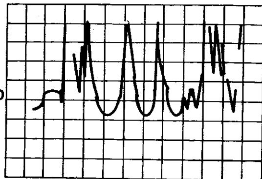
Figure 15. Variations of flywheel acceleration/deceleration signal and derived roughness with increasingly lean mixtures. (1200 rpm)
