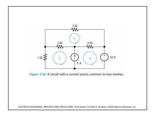
Combine meshes 1 and 2 into a **supermesh**. In other words, we write a KVL equation around the periphery of meshes 1 and 2 combined.
