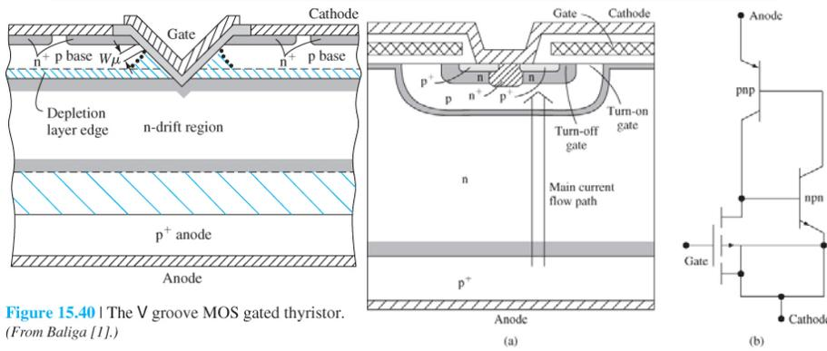
Figure 15.40 | The V groove MOS gated thyristor. (From Baliga [1].)
