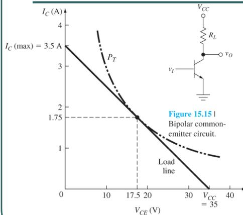
Figure 15.16 | Load line and maximum power curve for Example 15.1.
