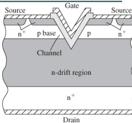
Figure 15.21 | Cross section of a vertical channel MOS (VMOS) transistor.
