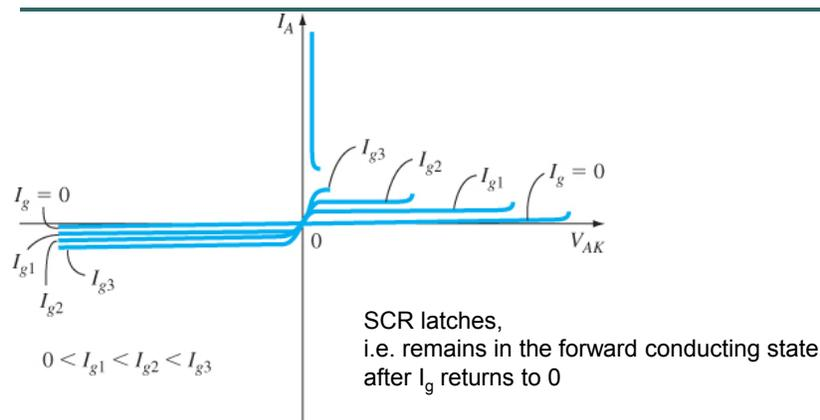
Figure 15.34 | Current-voltage characteristics of an SCR.
