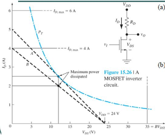
(a)  $BV_{DSS} = V_{DD} = 24\text{ V}$
