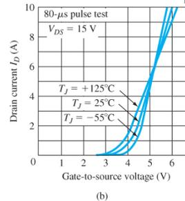
Figure 15.24 | Typical characteristics for high-power MOSFETs at various temperatures: (a) transconductance versus drain current; (b) drain current versus gate-to-source voltage. Note  $I_D$  decr with  $T$  incr at high  $V_{GS}$ .
