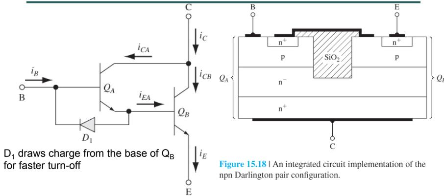
$D_1$  draws charge from the base of  $Q_B$  for faster turn-off
