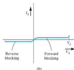
Figure 15.291 (a) The basic four-layer pnpn structure. (b) The initial current-voltage characteristic of the pnpn device.
