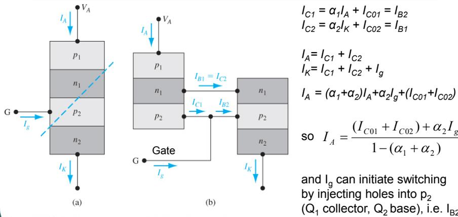
Figure 15.33 | (a) The three-terminal SCR. (b) The two-transistor equivalent circuit of the three-terminal SCR.
