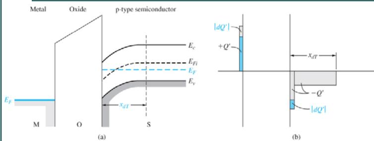
Figure 10.25 | (a) Energy-band diagram through a MOS capacitor for the inversion mode. (b) Differential charge distribution at inversion for a low-frequency differential change in gate voltage.
