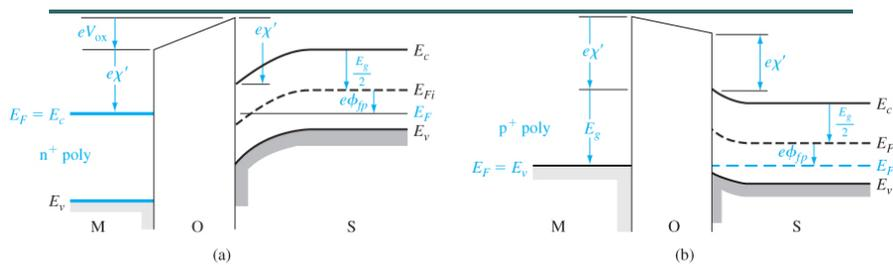
**Figure 10.14** | Energy-band diagram through the MOS structure with a p-type substrate at zero gate bias for (a) an n<sup>+</sup> polysilicon gate and (b) a p<sup>+</sup> polysilicon gate.
