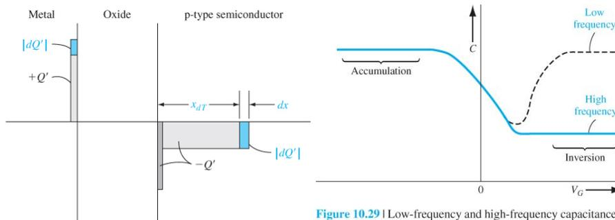
Figure 10.28 | Differential charge distribution at inversion for a high-frequency differential change in gate voltage.
