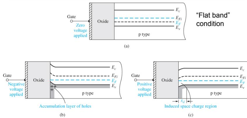
**Figure 10.4** | The energy-band diagram of a MOS capacitor with a p-type substrate for (a) a zero applied gate bias showing the *ideal* case, (b) a negative gate bias, and (c) a moderate positive gate bias.
