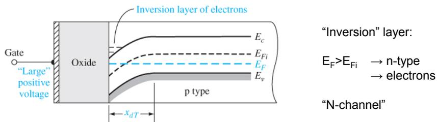
**Figure 10.5** | The energy-band diagram of the MOS capacitor with a p-type substrate for a "large" positive gate bias.
