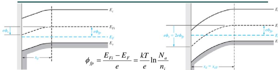
**Figure 10.8** | The energy-band diagram in the p-type semiconductor, indicating surface potential.
