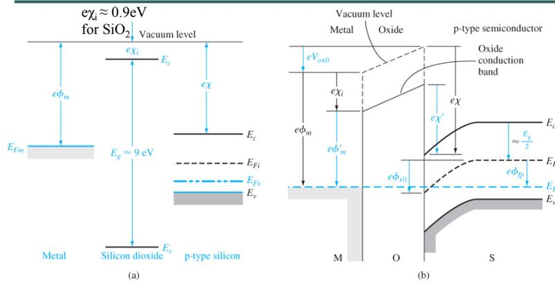
Figure 10.13 | (a) Energy levels in a MOS system prior to contact and (b) energy-band diagram through the MOS structure in thermal equilibrium after contact.
