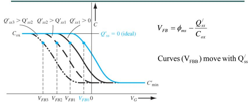
**Figure 10.30** | High-frequency capacitance versus gate voltage of a MOS capacitor with a p-type substrate for several values of effective trapped oxide charge.
