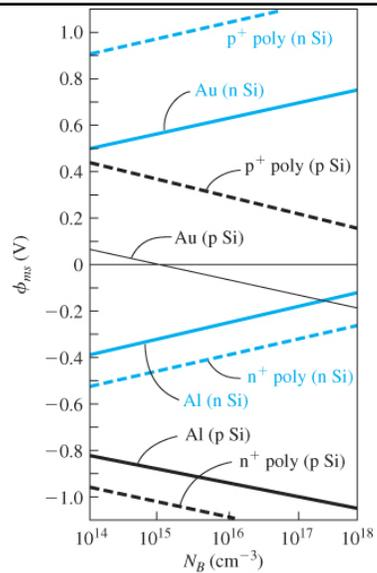
Figure 10.16 | Metal–semiconductor work function difference versus doping for aluminum, gold, and n<sup>+</sup> and p<sup>+</sup> polysilicon
