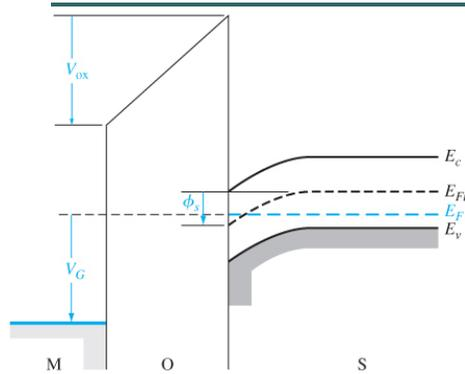
Figure 10.20 | Energy-band diagram through the MOS structure with a positive applied gate bias.
