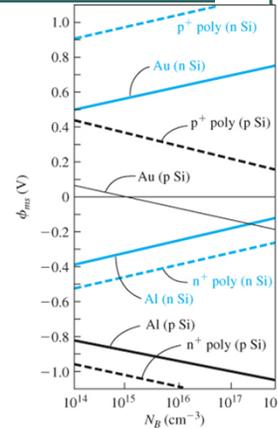
Figure 10.16 | Metal-semiconductor work function difference versus doping for aluminum, gold, and n<sup>+</sup> and p<sup>+</sup> polysilicon gates. (From See [17] and Werner [20].)
