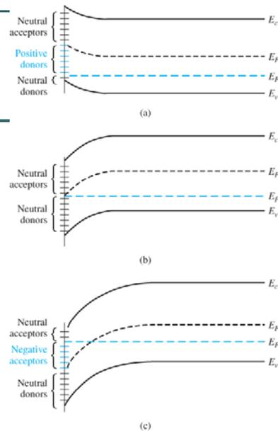
**Figure 10.32** | Energy-band diagram in a p-type semiconductor showing the charge trapped in the interface states when the MOS capacitor is biased (a) in accumulation, (b) at midgap, and (c) at inversion.
