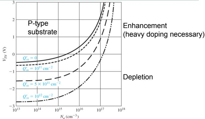
Figure 10.21 | Threshold voltage of an n-channel MOSFET versus the p-type substrate doping concentration for various values of oxide trapped charge ( $t_{ox} = 500 \text{ \AA}$ , aluminum gate).
