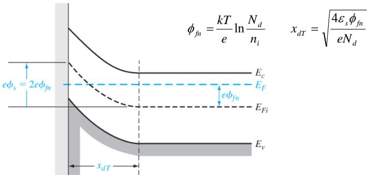
Figure 10.10 | The energy-band diagram in the n-type semiconductor at the threshold inversion point.
