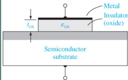
**Figure 10.1** | The basic MOS capacitor structure.
