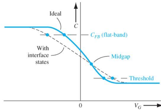
**Figure 10.33** | High-frequency C-V characteristics of a MOS capacitor showing effects of interface states.
