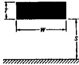
Fig E5 Cross-section of a microstrip line
