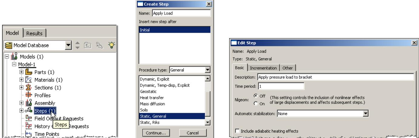
12. Expand the Field Output Requests node in the model tree, and then double click on F-Output-1 (F-Output-1 was automatically generated when creating the step)
