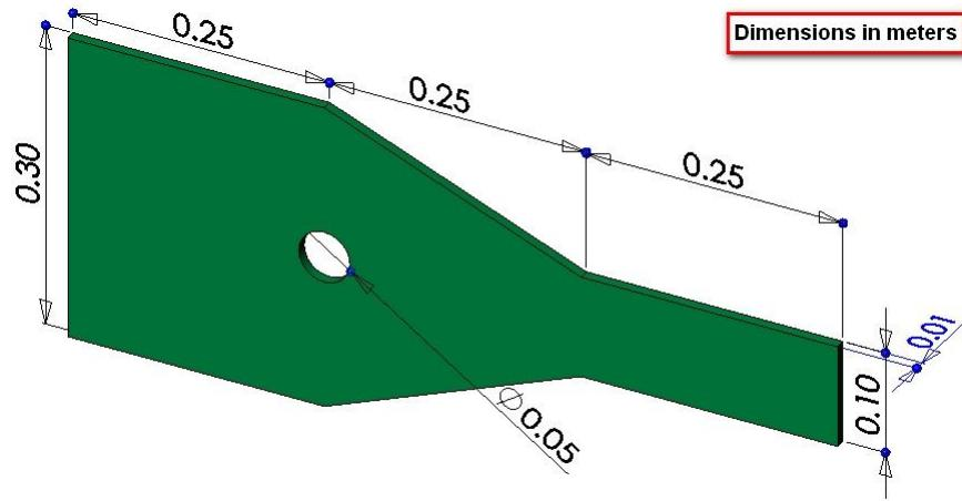
The steel bracket is fixed to a wall along its left side. A tensile pressure force with a total magnitude of 5000 N is applied to the right side of the bracket. The bracket contains one line of symmetry, so only half of the geometry is to be modeled. Determine the stresses in the bracket.
