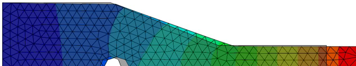
The image was obtained using the “superimpose options” icon and setting the parameters as shown. Note the clear stretching of the right side of the bracket and the imposition of symmetry BC preventing the lower horizontal segment from moving in the vertical direction.
