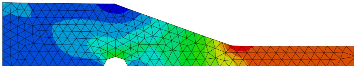
25. Request displacement plot along x-dir. With the undeformed shape superimposed.
