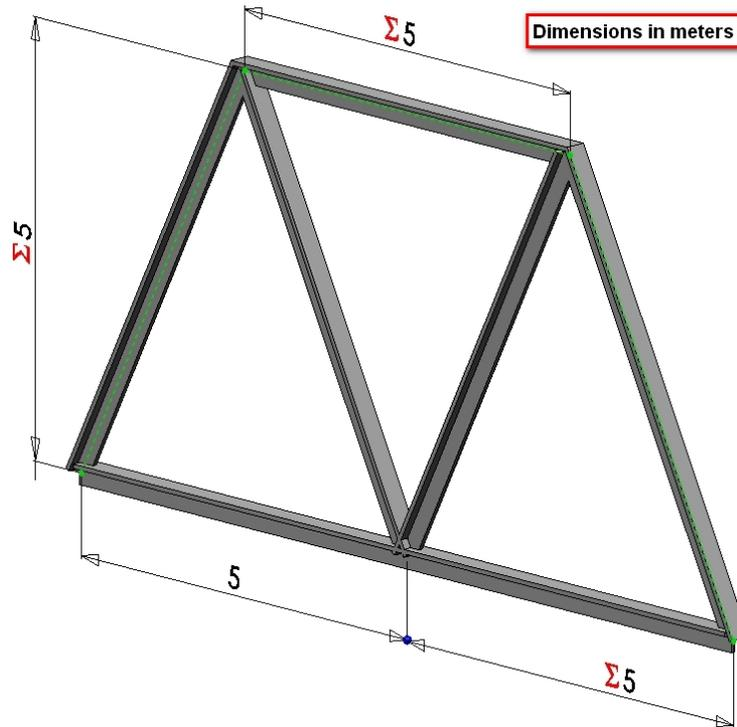
The two dimensional bridge structure, which consists of steel T-sections, is simply supported at its lower corners. Determine the first 10 eigenvalues and natural frequencies.
