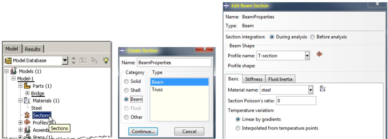
8. Expand the “Parts” node in the model tree, expand the node of the part just created, and double click on “Section Assignments” or use the “Assign Section” icon shown below
