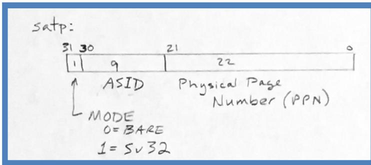
For RV64 systems, the **satp** register is 64 bits, arranged as follows:
