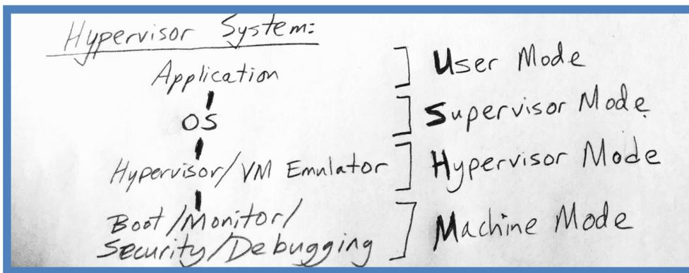
In the above diagrams we suggest which modes will be used for which sorts of code, but this is not mandatory. In particular, an operating system kernel might run in Machine Mode in some systems and in Supervisor Mode in other systems.
