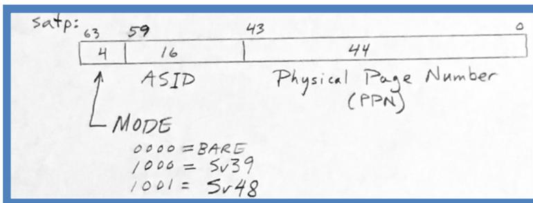
The MODE field indicates whether virtual memory address translation is turned on or not and, if so, which paging table scheme is being used.
