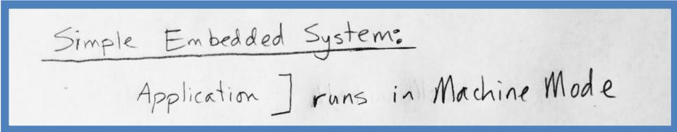
With option 2, there are two privilege levels: User and Machine. This might be appropriate for a simple OS with some protected security monitor running in Machine Mode and one or more applications running in User Mode.
