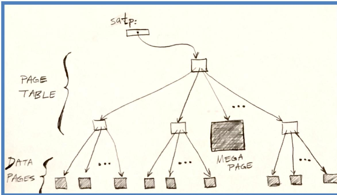
There is a facility for “megapages”. A megapage is a data page containing 4 MiBytes. An offset into a megapage will be 22 bits, since  $2^{22} = 4 \times 1,024 \times 1,024 = 4,194,304$ . A megapage must be aligned to a 4 MiByte boundary.
