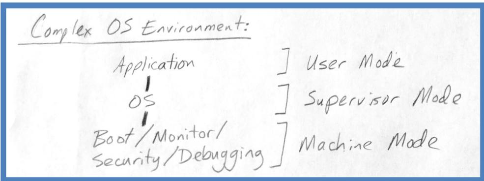
In some implementations several instructions and/or ISA features will be missing and there will be a need to emulate the missing functionality. The natural organization will place the code to emulate the missing instructions/features in Machine Mode so that the OS (which runs in Supervisor Mode) does not need to be aware of these details.
