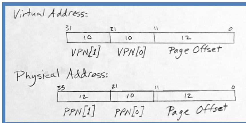
The size of each page is 4,096 bytes, and each byte within a page can be addressed by 12 bits, since  $2^{12} = 4,096$ . All pages must be properly aligned on a 4,096 byte boundary.
