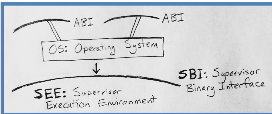
The OS might be running on bare metal. Or the OS might be running on top of a hypervisor or some other monitor/security/bootstrapping software. In any case, the OS is created and written to meet the specifications of a “Supervisor Execution
