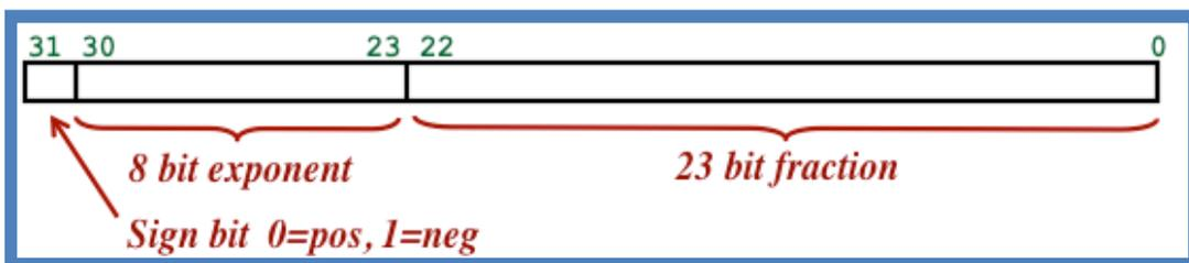
Let  $N$  be the number represented. Let “**sign**” be the most significant bit. Let “**exponent**” be the bit pattern in bits 30:23. Let “**fraction**” be the bit pattern in bits 22:0.
