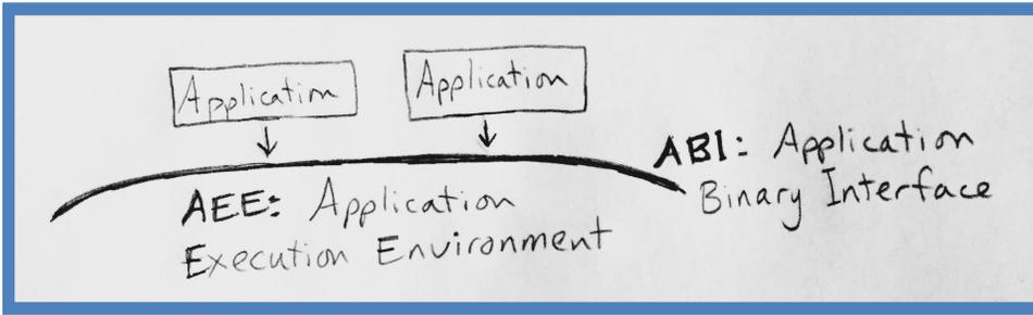
Typically an OS sits underneath the application and implements the Application Binary Interface, which consists of the User Mode instruction set along with the collection of system calls that are available to applications. The Application Binary Interface is the sum total of what the application programmer needs to understand in order to write programs; the programmer does not have to understand or know what is going on within the Application Execution Environment.
