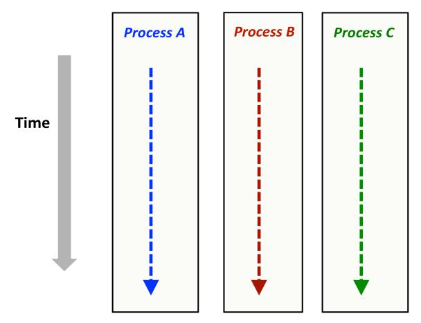
Finally, we move out even further. At this point, the time-slices are no longer visible and we can see the entire process execution, from process creation to process termination. In this view, it appears that all processes are executing with true concurrency, although you now know this is an illusion.
