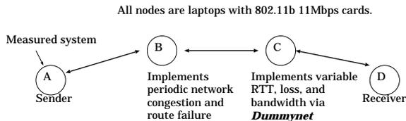
Figure 3: Measurement setup.
