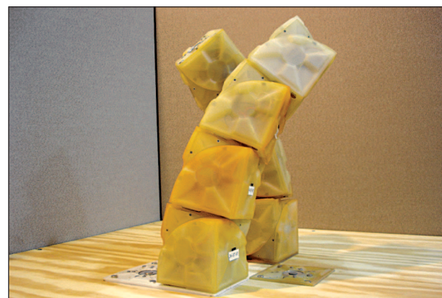
FIGURE 8 Zykov, Mytilinaios, Adams, and Lipson's self-replicating robot and a copy (photo courtesy of Cornell University).
