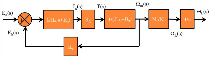
Motor position transfer function with speed changer. Note:
