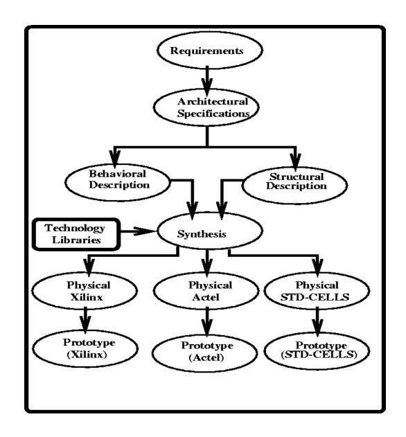
Fast prototyping is done in reprogrammable FPGAs (Xilinx) or OTP FPGAs (Actel). The final verified design is often implemented using standard cells.
