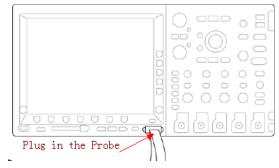
2. Connect the desired logic probe tips to desired test points on your circuit, for example, CLK or DATA bus; Please remember to connect the **GROUND** pin;
