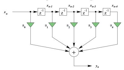
The input to this filter is a sequence  $\{x_0 \ x_1 \ x_2 \ \ldots\}$  which results in an output response  $\{y_0 \ y_1 \ y_2 \ \ldots\}$  where
