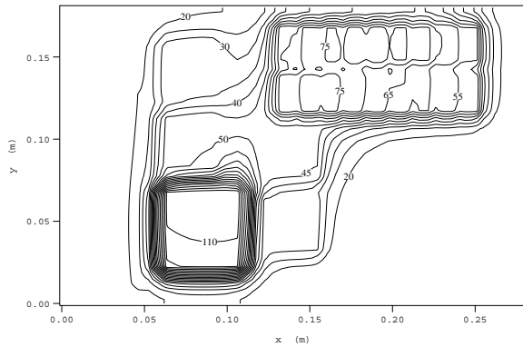
Figure 9: Temperature contours in a plane 0.19 cm from the bottom of the domain. The temperature field is computed on a 57 \times 34 \times 37 grid.
