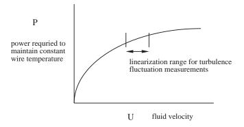
Each probe must be calibrated. A working formula of the form
