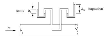
If the fluid in the duct is a gas, then the pressure change due to elevation differences  $in\ the\ gas$  is negligible. In this case the manometer attached to the static pressure tap measures
