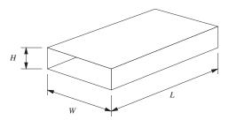
For fully-developed flow in a duct, the flow regime is determined by the Reynolds number based on hydraulic diameter
