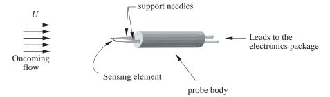
A typical system uses a wire made of tungsten or platinum that is approximately 1 mm long and 5  $\mu$ m in diameter. The wire is attached to support needles that provide physical support and electrical connection to the output electronics. The probe can be detached from the support structure that is used to position the probe in the flow. Hot wire probes are very delicate and any planned experiment must include a budget for replacement and repair of probes.
