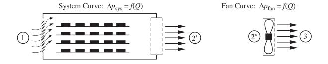
On the left, station 2' is the exit pressure necessary to draw the a given flow rate through the system when the fan is not powered. On the right, station 2'' is the upstream condition for the fan during a fan test, i.e., when the fan is not connected to a system.
