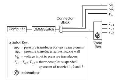
Figure 2: Block diagram for flow bench instrumentation
