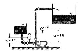
Calculate the net head delivered and the pump efficiency at a volume flow rate of 1000 gpm. Plot the pump head, power, and efficiency as functions of volume flow rate
