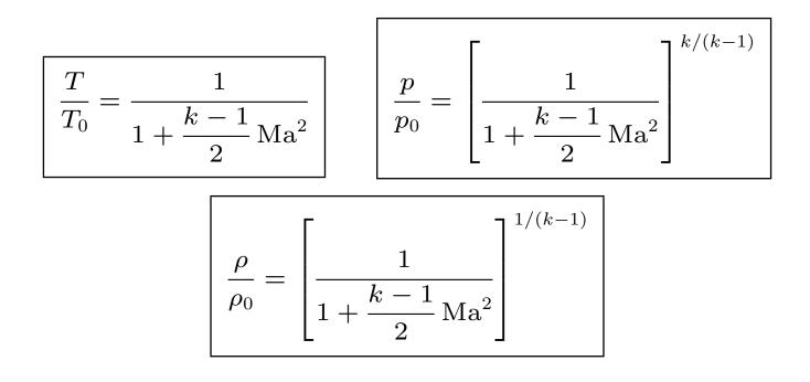
Given Ma it is straightforward to find  $T/T_0$ , but given  $T/T_0$  an iterative root-finding procedure is necessary to compute Ma. These equations are tabulated so that it's possible to work them in both directions. See Munson, Young, and Okiishi, Figure D.1, p. 7.66
