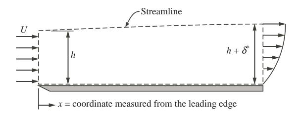
$\delta^*$  is the amount by which the streamline just outside the boundary layer is displaced.
