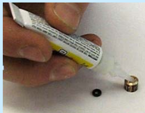
STEP 5: glue in o-ring
