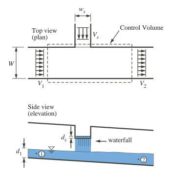
You have paid a consultant to perform some measurements on the water velocity in the ditch. The consultant reports that the velocity at station 2 is the same as station 1, i.e.  $V_2 = V_1$ . A co-worker tells you that because of the flow from the side channel,  $V_2$  cannot be equal to  $V_1$ .
