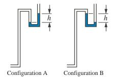
b. [17 points] What is the value of h if  $p_{\rm in}$ ,  $V_{\rm in}$ , d, D, and L are known? Assume that the velocity is uniform across the duct at any cross section. Start with basic equations governing the flow and develop a formula for h.
