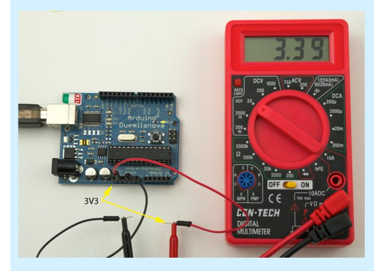
If you need less than 5V for a project, you can use the 3V3 pin, Which provides about 3.3V. The current draw from the 3V3 pin is limited to 50mA.
