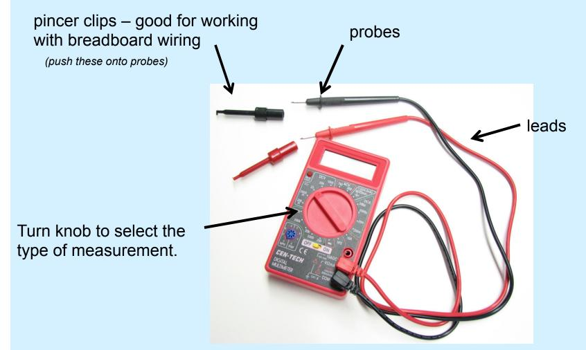
You will use the multimeter to understand and troubleshoot circuits, mostly measuring DC voltage, resistance and DC current.
