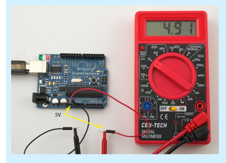
The measured voltage is close to 5V target.
