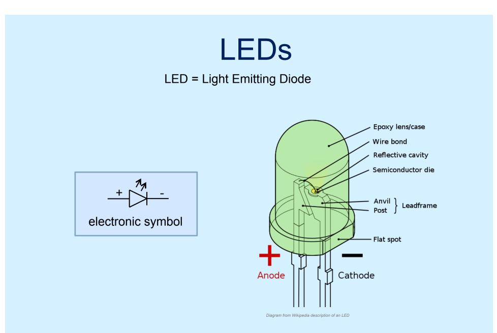
Electricity can only flow one way through an LED (or any diode). The flat spot on the LED must be connected to ground (GND).
