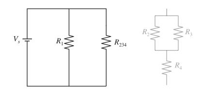
$R_1$  and  $R_{234}$  can be further combined to give the equivalent resistance for the circuit
