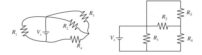
Use  $R_1=R_2=330\,\Omega$ ,  $R_3=500\,\Omega$ ,  $V_s=12\,\mathrm{V}$  and let  $R_4$  vary from  $50\,\Omega$  to  $500\,\Omega$ .
