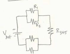
$$R_{345} = R_3 + R_4 + R_5$$
