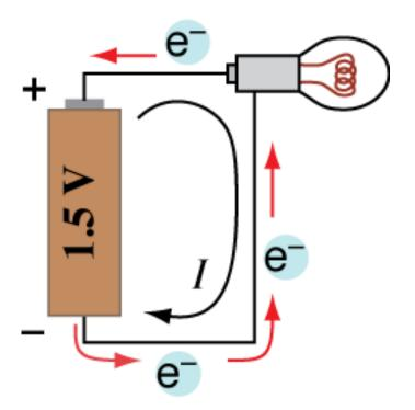
A 1.5 volt AA battery is wired to a light bulb with a resistance of 30  $\Omega$ .
