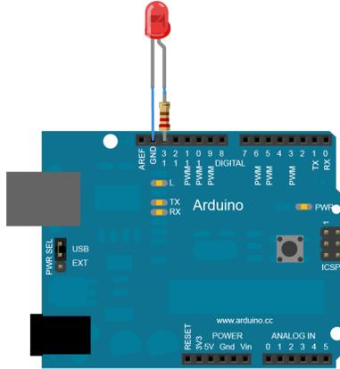
Schematic of the blink circuit from <http://www.arduino.cc/en/Tutorial/Blink>
